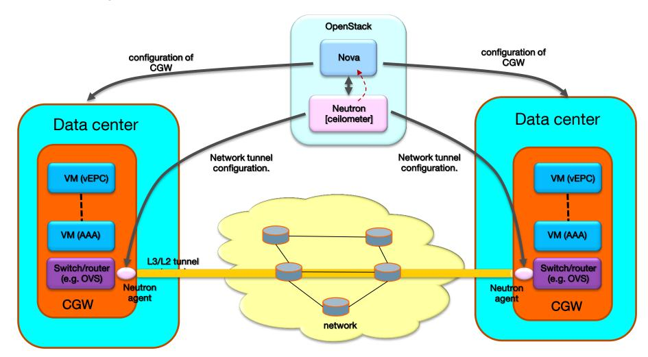
Openstack can control and configure a CGW from the edge (nothing in the network)
